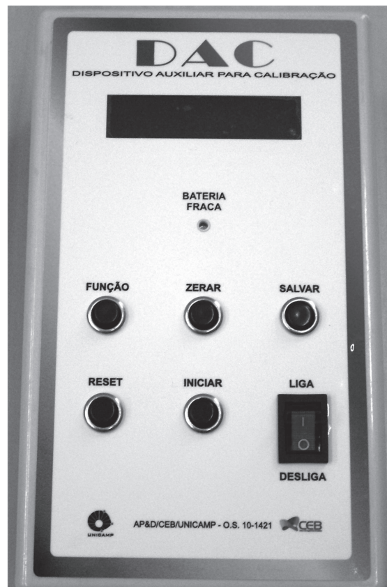
Fig. 3 - Photographic record of the assistive device for calibration (ADC) used for measurements of mean pressure of dynamic calibration
