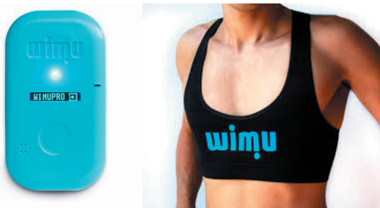
Figure 1. (a) Image of the WIMU PRO™ inertial device and (b) anatomical adjusted harness in one of the study participants.
