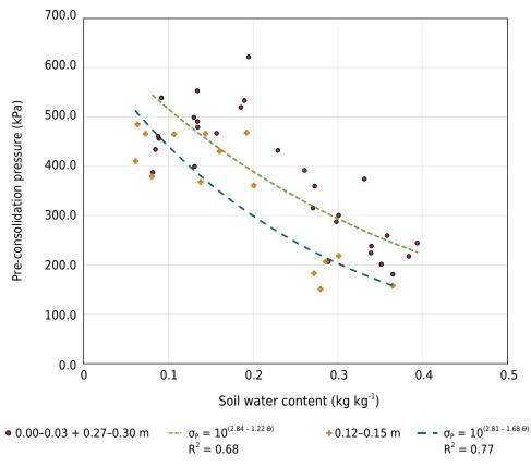
Figure 3. Load-bearing capacity model of shaded treatment after grouping data from the 0.00-0.03 and 0.27-0.30 m layers.
