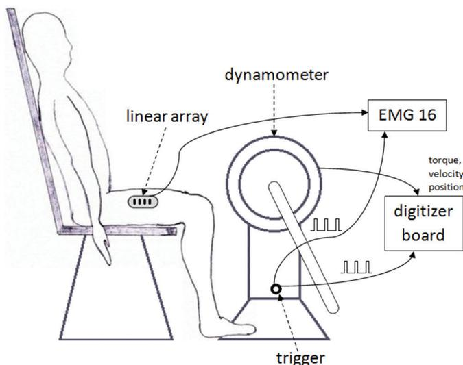
Figure 2. Instrumentation architecture.
