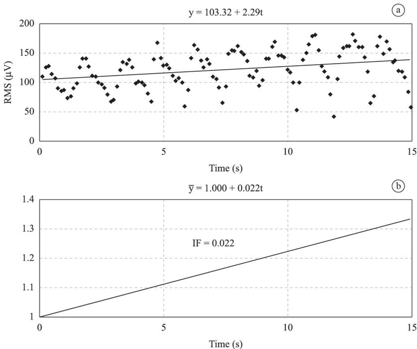
Figure 3. (a) Linear regression for the RMS parameter and (b) the respective index of fatigue (IF).
