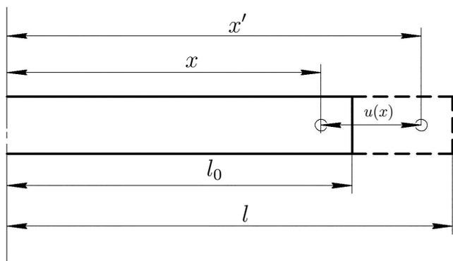
Figure 2: The geometric characteristics of the elongation deformation.
