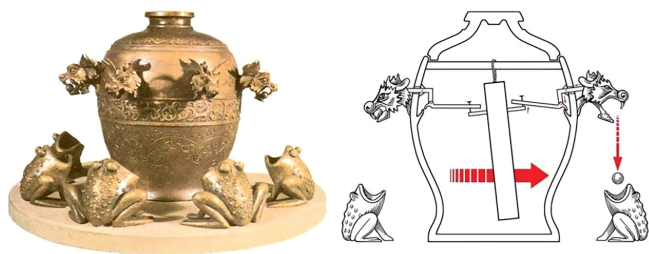
Figure 1: Chinese seismograph invented by the scientist Zhang Heng (78–139 AD), the cylindrical rod-shaped pendulum inside oscillates during an earthquake [4].
