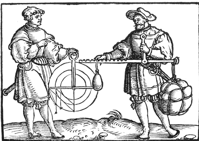
Figure 4: An illustration of the Roman balance (or statera ), a common instrument used for the study of equilibrium by Renaissance philosophers [12, p. 62].
