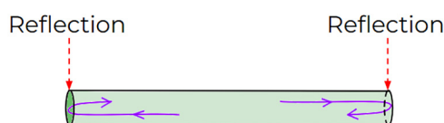
Figure 5: In this model, the pressure wave reflects at both ends, so it is trapped in a finite space.
