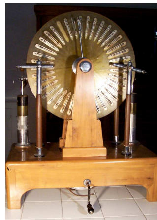
Figura 6 - One of a twin couple of electrostatic machines signed "Vittorio Ugobono" placed in "Istituto Gianelli" in Chiavari. Disk diameter 460 mm. Other twin unfinished machine (without Leyden jar) is placed in a private collection. Another machine found near Chiavari (and now in a private collection) has disks with the same typical sectors but a very different style in wood construction.
