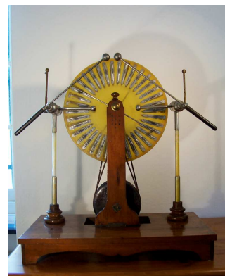
Figura 1 - Wimshurst electrostatic machine (unsigned) placed at Museo di Fisica e meteo-sismologia “G. Sanguineti-G. Leonardini”. Thin foil sectors come from the mould used in the Caranza workshop (after Caranza’s death, this workshop was take over by V. Ugobono). Glass disk have diameter 400 mm. This machine appears as a merge of parts coming from different previous machines: part of the metallic structure in brass and part in chromium plated brass.
