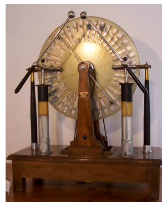
Figura 2 - Wimshurst electrostatic machine (signed Egidio Caranza) placed in Museo di Fisica e meteo-sismologia “G. Sanguineti-G. Leonardini”. Thin foil sectors differs from the standard of this maker. Glass disk have diameter 480 mm. As the previous machine, these apparatuses were used in the Physics Cabinet of (Seminario Vescovile) where not only Religious but also laymen studied from 1828 up to end of the XIX century. From a photographic comparison with old photographic documentation before restoration, sectors are original as the double presence of brass and chromium plated brass in both machines.
