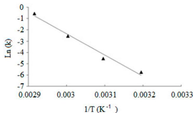
**Figure 6.** The graphical representation of Arrhenius for ICg.
