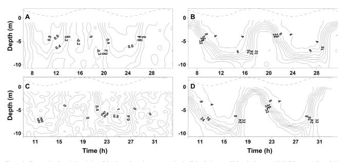
Figure 3 - Temporal and vertical variation of the along-channel current speed and salinity during two tidal cycles between 18-19 February (A,B) and 16-17 July (C,D). Positive current velocity means downstream and negative means upstream.
