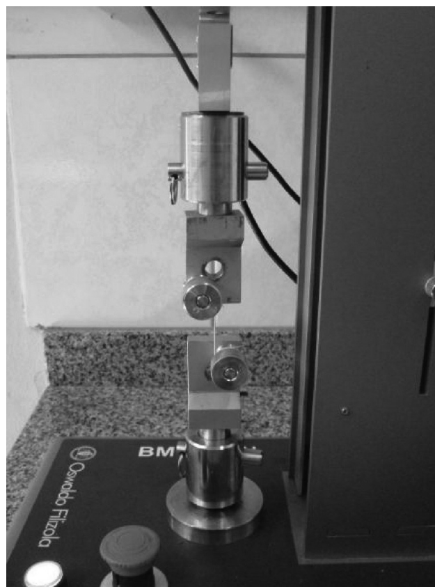
Fig. 3 Metallic claw for assays with sutures at an initial length of 5 cm.
