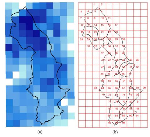
Figure 4. a) Discrete radar reading and b) Pixels influencing the basin (673.6x673.6 m).
