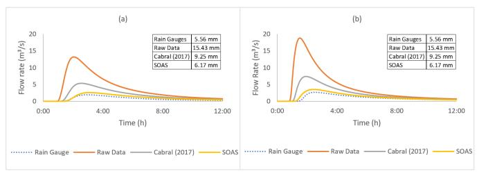
Figure 10. Hydrographs day 02/02/2019: a) Concentrated and b) Distributed.
