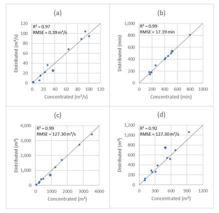
Figure 6. Comparison between the parameters of the evaluated scenarios: a) Peak flow, b) Peak time, c) Flowed volume and d) Inlet volume.
