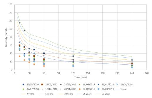
Figure 3. Estimation of the return periods of the selected events, for each duration, considering the IDF curve of Pfafstetter (1957) for Maceió.
