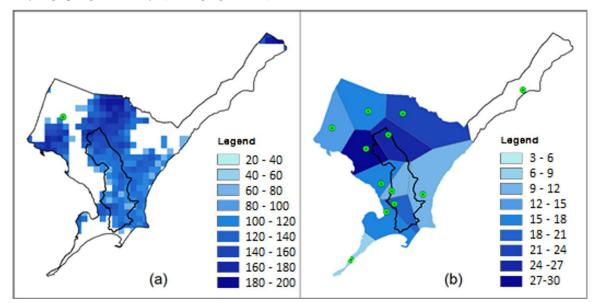
Figure 13. Readings for the same period of time: a) Radar and b) rain gauges (subtitles in mm).
