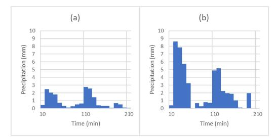
Figure 12. Hyetographs generated by: a) Rain gauges and b) Raw radar data.
