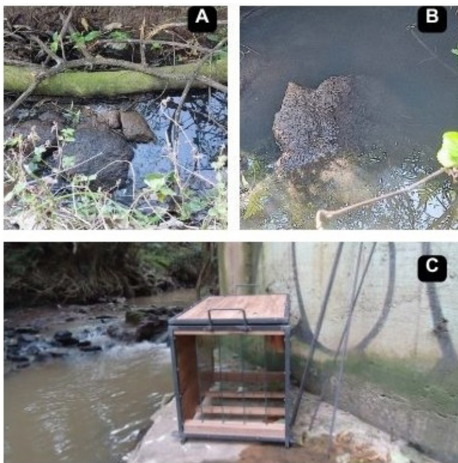
Figure 2. Sampler examples. A and B represent natural samplers, while C represents an artificial sampler. A - Piece of tree trunk with natural biofilms on top (wood). B – Stone full of natural biofilm. C - wooden box with internal glass sheets, to be submerged in the river, for biofilm adhesion.
