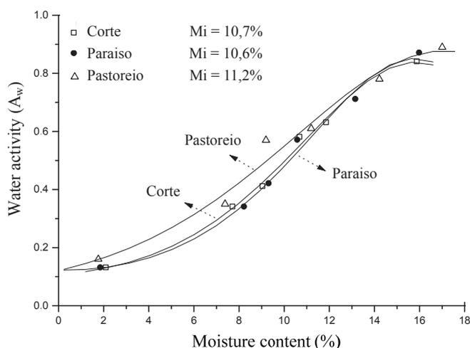
Figure 2. Sorption and desorption isotherms at 25 °C for seed of three different interspecific hybrids (*Pennisetum purpureum* x *Pennisetum glaucum*): Paraiso, Corte and Pastoreio. ( $M_i$  - initial moisture content).
