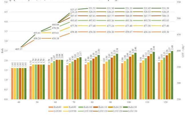
Figure 8 - Variations in Nominal Yield (NY) and Field Productivity (TCH) and its impacts on the loading–harvester ratio (Ralh) and loading operational yield (LOY) in dual-row simultaneous harvest in 1.50 m spacing
