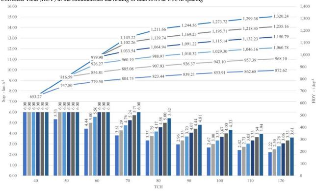
**Figure 4 -** Variations in Nominal yield (NY) and Field Productivity (TCH) and their impacts on Operating speed (Sop) and Harvester Corrected Yield (HCY) in the simultaneous harvesting of dual rows at 1.50 m spacing
