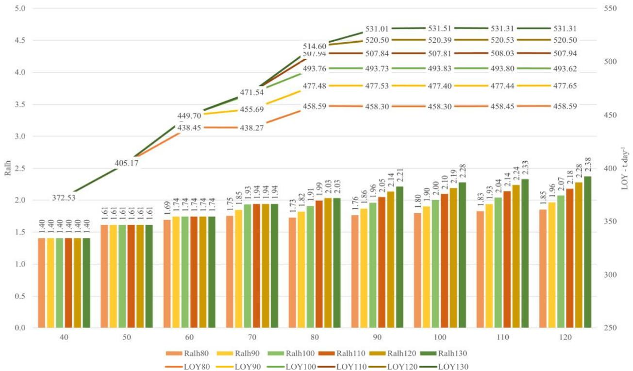
**Figure 8** - Variations in Nominal Yield (NY) and Field Productivity (TCH) and its impacts on the loading-harvester ratio (Ralh) and loading operational yield (LOY) in dual-row simultaneous harvest in 1.50 m spacing
