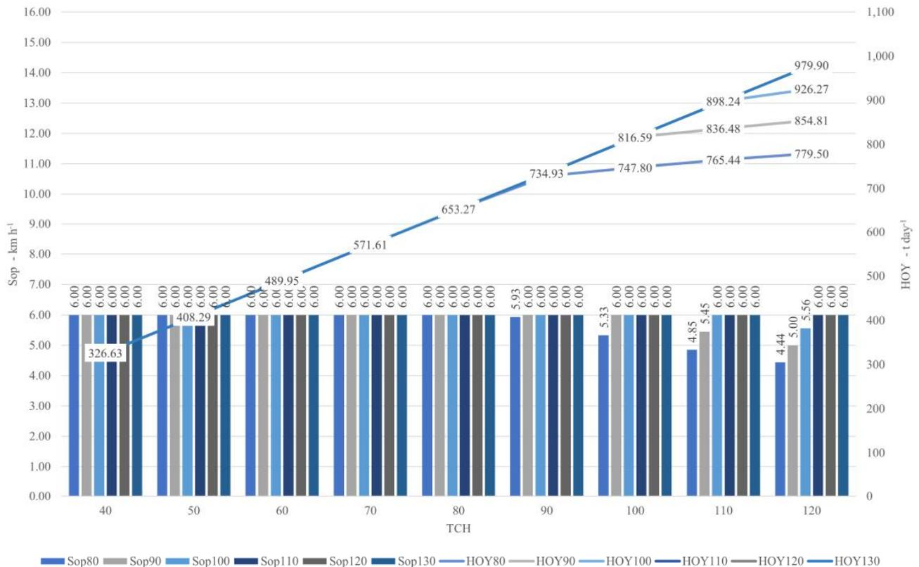
**Figure 2 -** Variations in Nominal yield (NY) and Field Productivity (TCH) and their impacts on Operating speed (Vop) and Harvester Corrected Yield (HCY) at 0.90 m x 1,40 spacing
