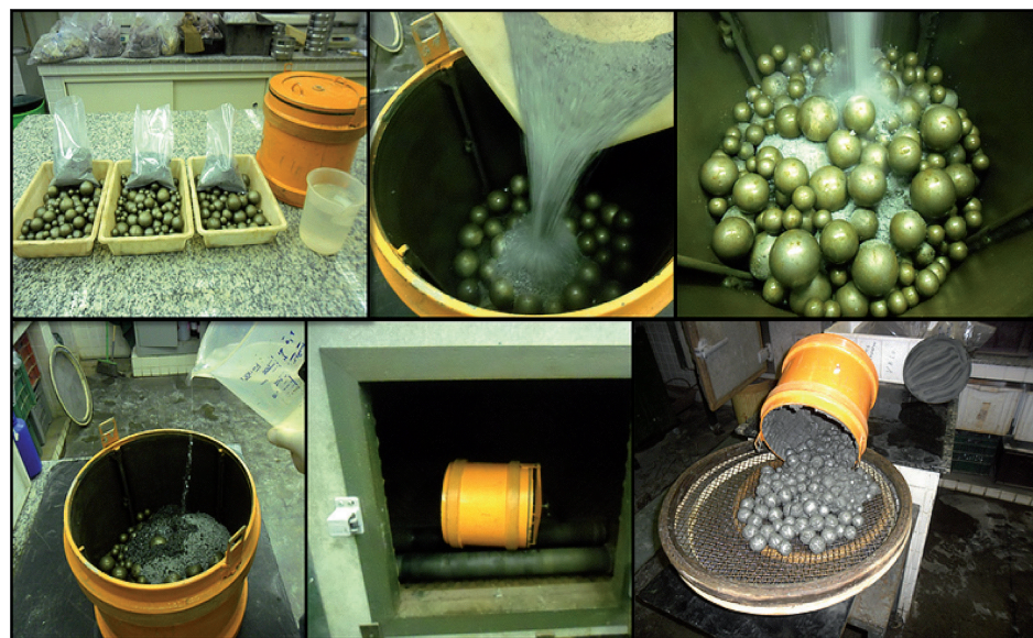
Figure 1 Test grinding ball mill sequential procedure.
