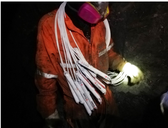
Figure 3 - Miner, wearing primed cartridges around his neck for transportation. Source: Universidad Adolfo Ibañez
