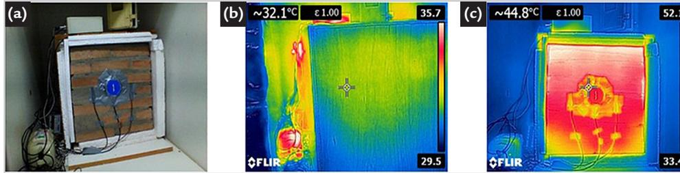
Figure 3 - (a) the panel with fluxmeter and temperature sensors, (b) assembled climate chamber and (c) photo of the panel obtained with the FLIR thermal imager after 72 hours of testing.
