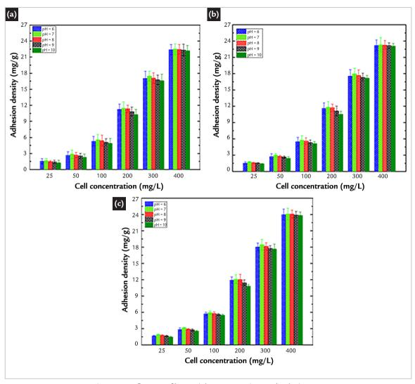
Figure 4 - Influence of bacterial concentration and solution pH on adhesion density at different temperature values: a)  $20^{\circ}$ C, b)  $30^{\circ}$ C and c)  $40^{\circ}$ C.
