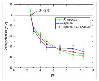
Figure 1 - Zeta potential curves of the *Rhodococcus opacus* bacteria and the apatite mineral (indifferent electrolytic: NaCl 10<sup>-3</sup> mol/L).
