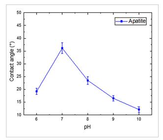
Figure 2 - Values of contact angle of the apatite mineral after interaction with the *R. opacus* bacteria. Cell concentration 100 mg/L and contact time of 5 minutes.
