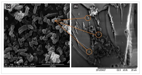
Figure 3 - SEM Images of the bacterial cells: a) *Rhodococcus opacus* cells and b) *Rhodococcus opacus* cells onto the apatite surface.
