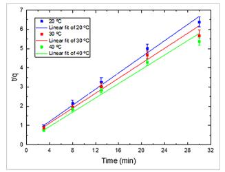
Figure 7 - Kinetics of *Rhodococcus opacus* adsorption onto apatite surface. The data were fitted using the pseudo-second order kinetic model.
