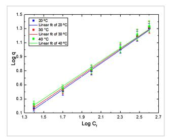
Figure 5 - Adsorption isotherm of *R*. opacus onto apatite surface. The data were fitted with *Freundlich* model (Temperature:  $20^\circ$ ,  $30^\circ$ ,  $40^\circ$  C).
