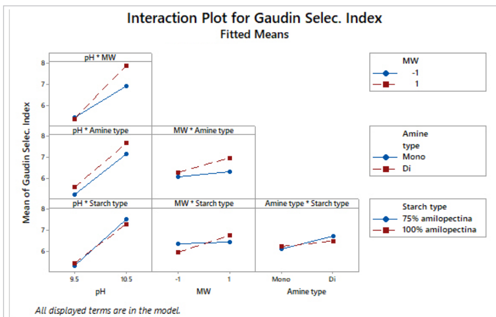
Figure 6 – Interaction of Gaudin selectivity index between pH, molecular weight, amine type and starch type.
