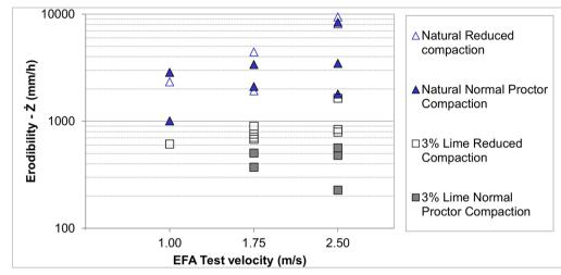
Figure 3 - Erodibility of natural and lime-treated soil samples, produced with reduced and Normal Proctor Compaction energies.
