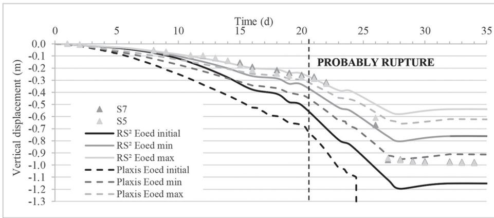
Figure 5 - Vertical displacements comparison.
