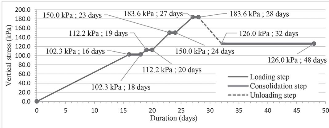
Figure 2 - Evolutionary sequence of loading in the test area.
