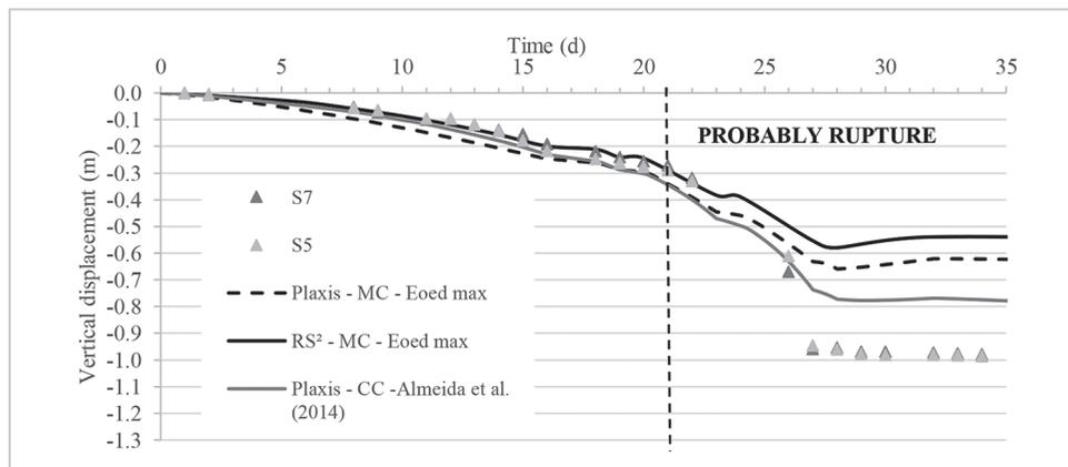
Figure 6 - Vertical displacements - Mohr Coulomb (MC) and Cam-Clay (CC) analysis.
