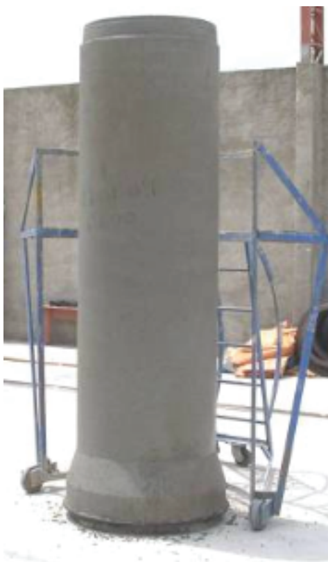
Figure 5 - General appearance of a new fiber reinforced concrete pipe
