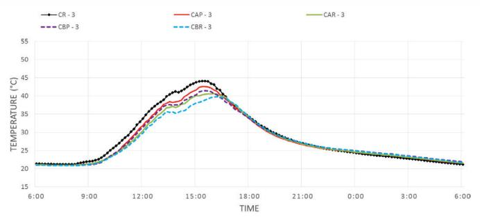
**Figure 6**Temperatures of sensors on bottom of slabs
