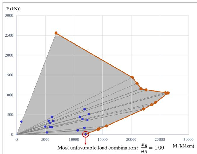
**Figure 18.** Interaction curve ( $P, M_y$ ) for 2C column.
