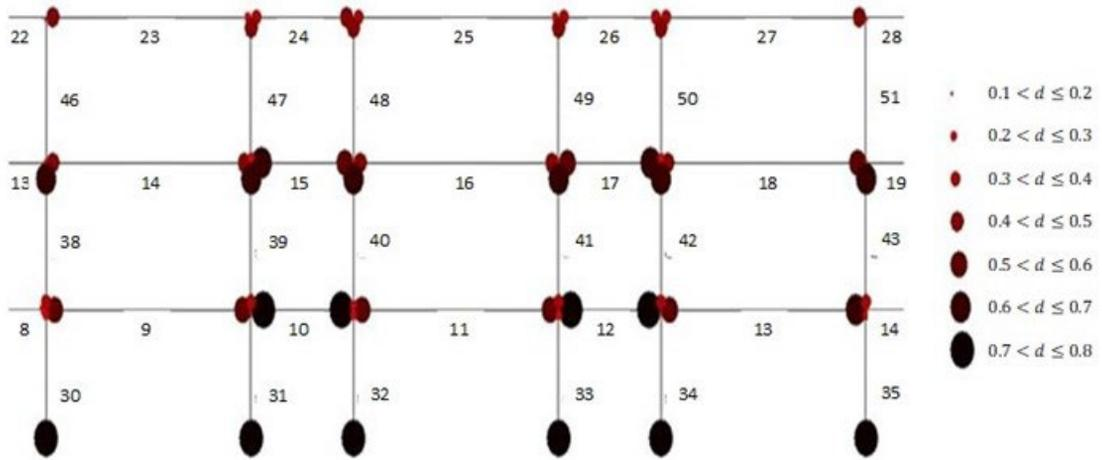
Figure 9. Example of plastic hinges in the LRMC transverse frame.
