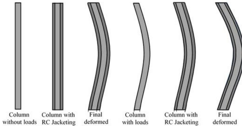
Figure 4. Columns deformed with and without preload.
