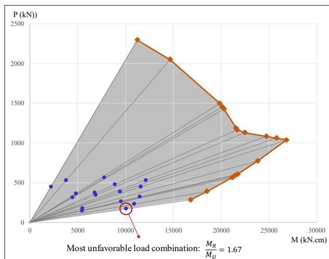
Figure 15. Interaction curve ( $P, M_x$ ) for 2B column.
