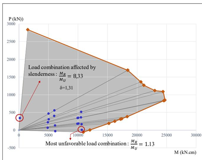
Figure 17. Interaction curve  $(P, M_x)$  for 2C column.
