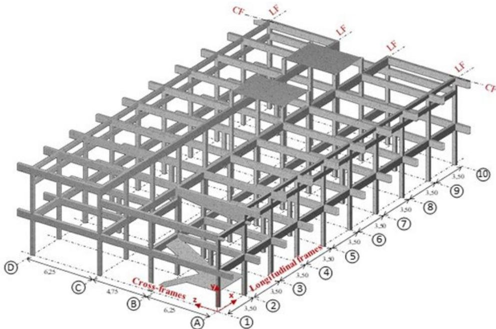
Figure 10. Building Structural System.
