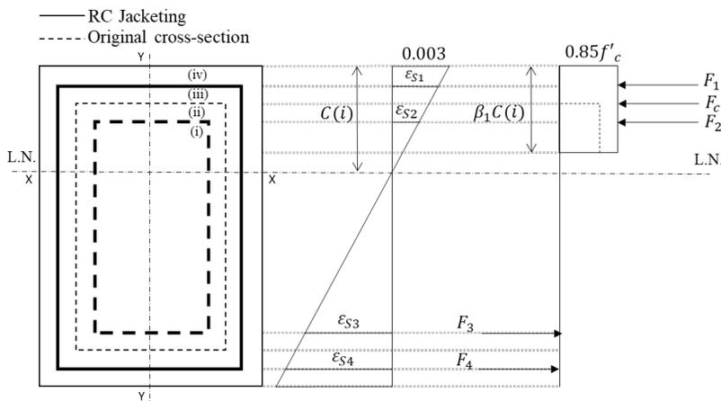
Figure 13. Diagram of deformations and internal forces in the section with RC Jacketing.
