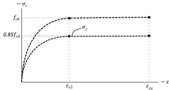
Figure 5. Idealized parabolic-rectangle stress-strain diagram for concrete.
