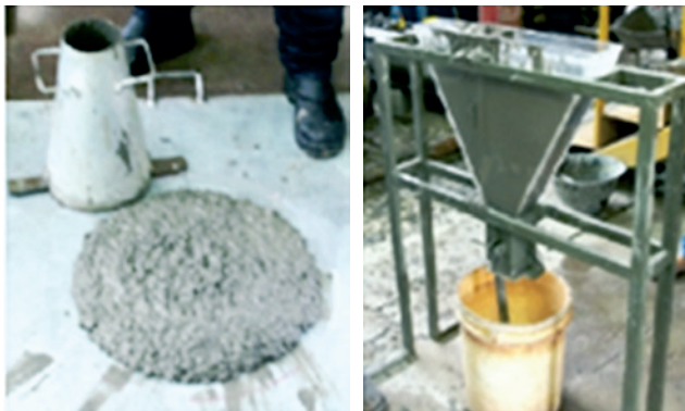
A Slump test
