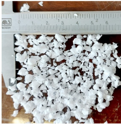
Figure 2. EPS waste used as lightweight aggregate.
