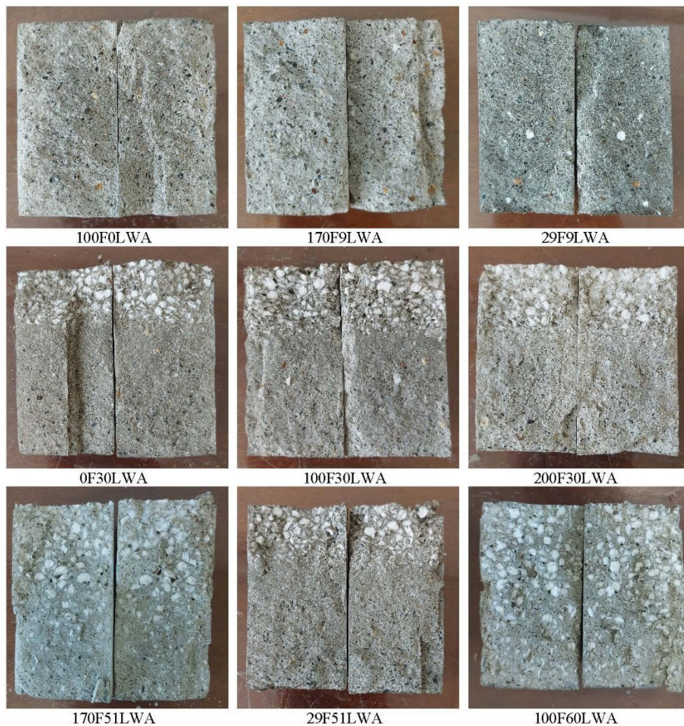
Figure 8. Images of the broken specimens obtained in the diametrical compression tests.
