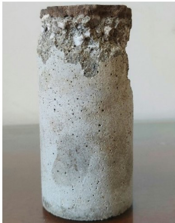
Figure 9. Specimen ruptured in the compressive strength test.
