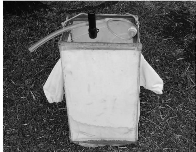
**Figure 1** - Quadrangular pyramidal trap (QP), especially developed to collect these insects in wild animal burrows
