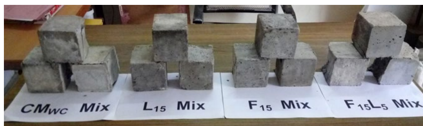
Figure 19: Visual appearance of the cubes after 180 days submergence in \text{MgSO}_4 solution.
