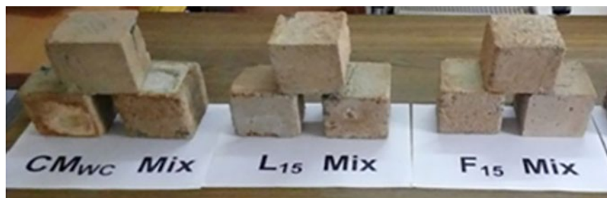
Figure 16: Visual appearance of the cubes after 180 days submergence in HCL acid solution.
