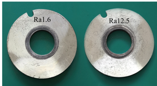
Figure 7: Comparison of wear of test pieces with different roughness.
