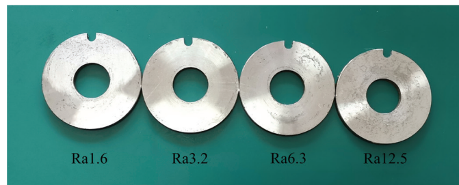
Figure 4: Test parts with different surface roughness.
