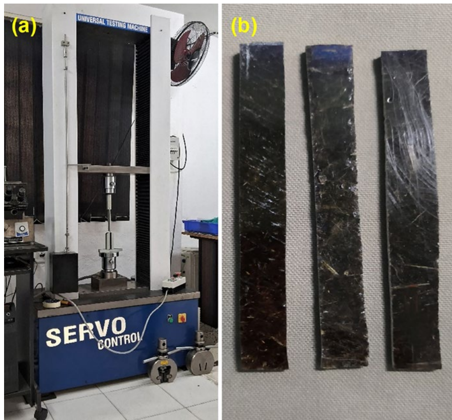
Figure 3: (a) Universal testing machine, (b) flexural test samples.
