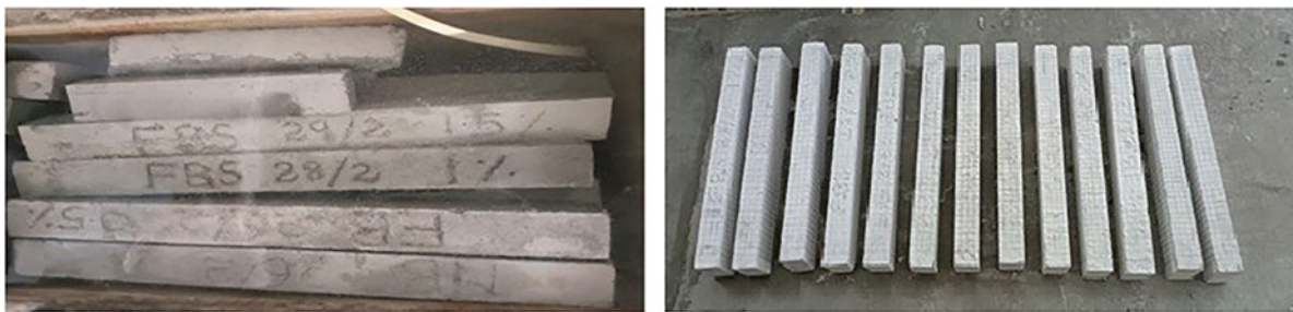
Figure 5: Curing and grit marked for all casted specimens.
