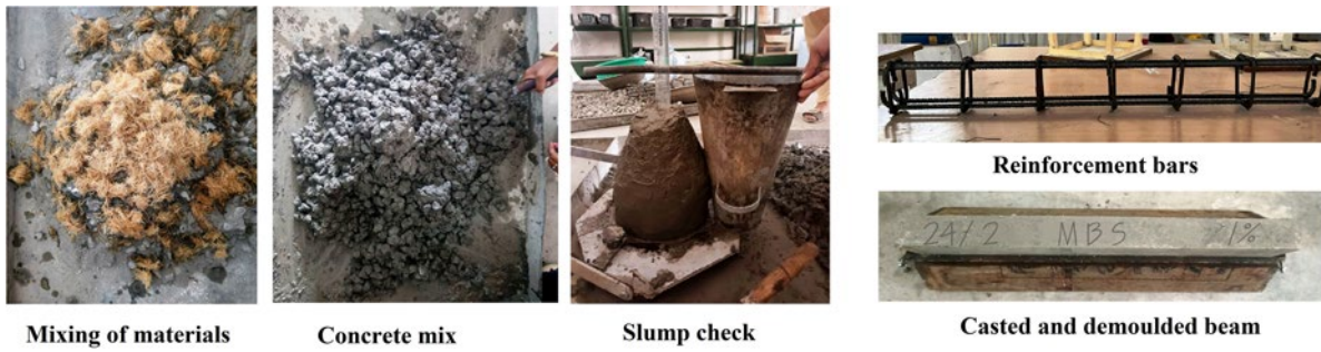
Figure 4: Manufacturing process of concrete.
