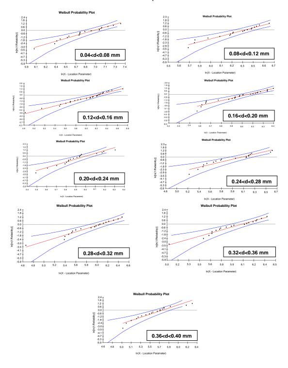
Figure 4: Weibull graphs for the tensile strenght of sisal fibers for different diameter intervals.
