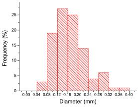
**Figure 2:** Statistical distribution of diameter of the sisal fibers for this work.
