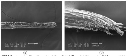
**Figure 7:** SEM fractograph of tensile-ruptured tips of sisal fibers (a) thinner, d = 0.05 mm and (b) thicker, d = 0.15 mm.
