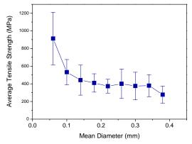
Figure 6: Variation of the average tensile strength with the mean diameter for sisal fibers.
