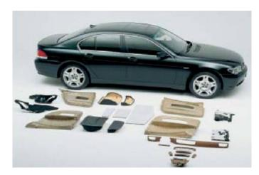
**Figure 1**: Components of a BMW sedan fabricated with lignocellulosic fiber reinforced polymer composites [5].
