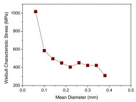
Figure 5: Variation of the characteristic strength with the mean diameter of sisal fibers.
