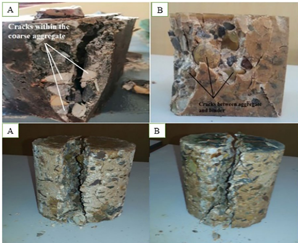
Figure 24: A- cracks in heat cured specimen, B- cracks in air cured specimen.
