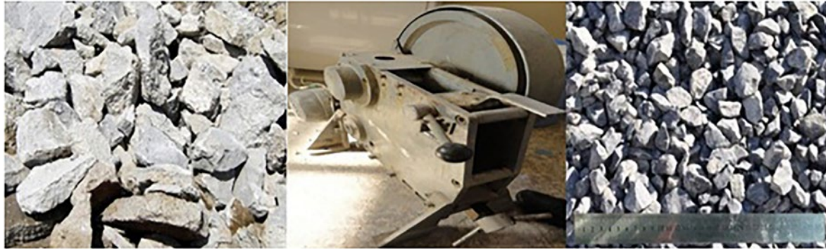
Figure 5: Crushing process of the recycle aggregate.
