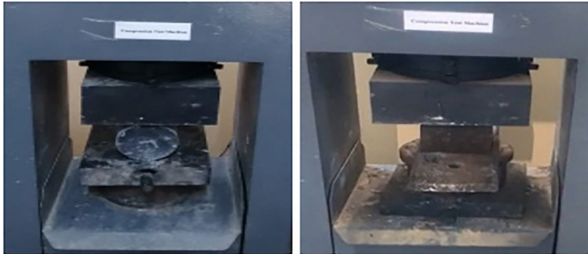
Figure 10: Splitting tensile test at the right and compressive test at the left.
