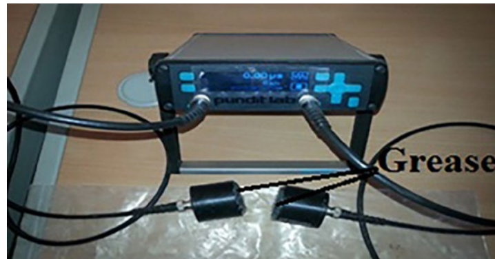
Figure 12: Ultrasonic pulse velocity apparatus used in the work.
