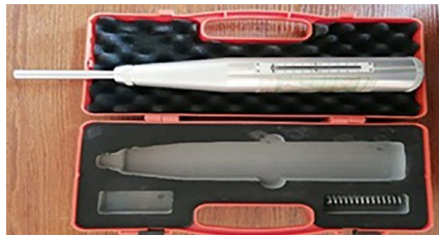
Figure 11: Schmidt hammer apparatus used in the work.
