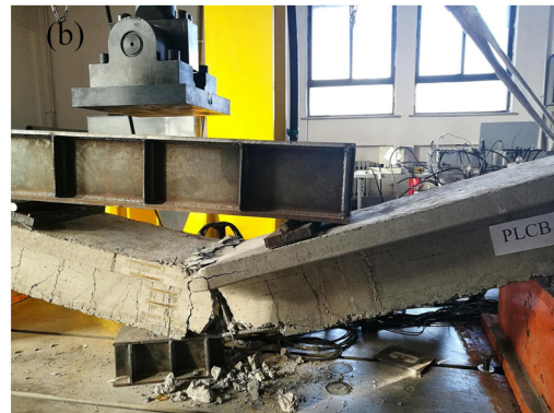
Figure 9: Failure mode of beam PLCB under fatigue load. (a) Curve of midspan deflection and number of cycles; (b) Steel bar fracture diagram of the beam PLCB.
