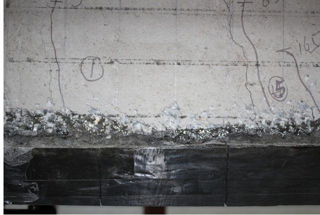
Figure 17: Failure mode of beam PLB2 under static load after fatigue test.
