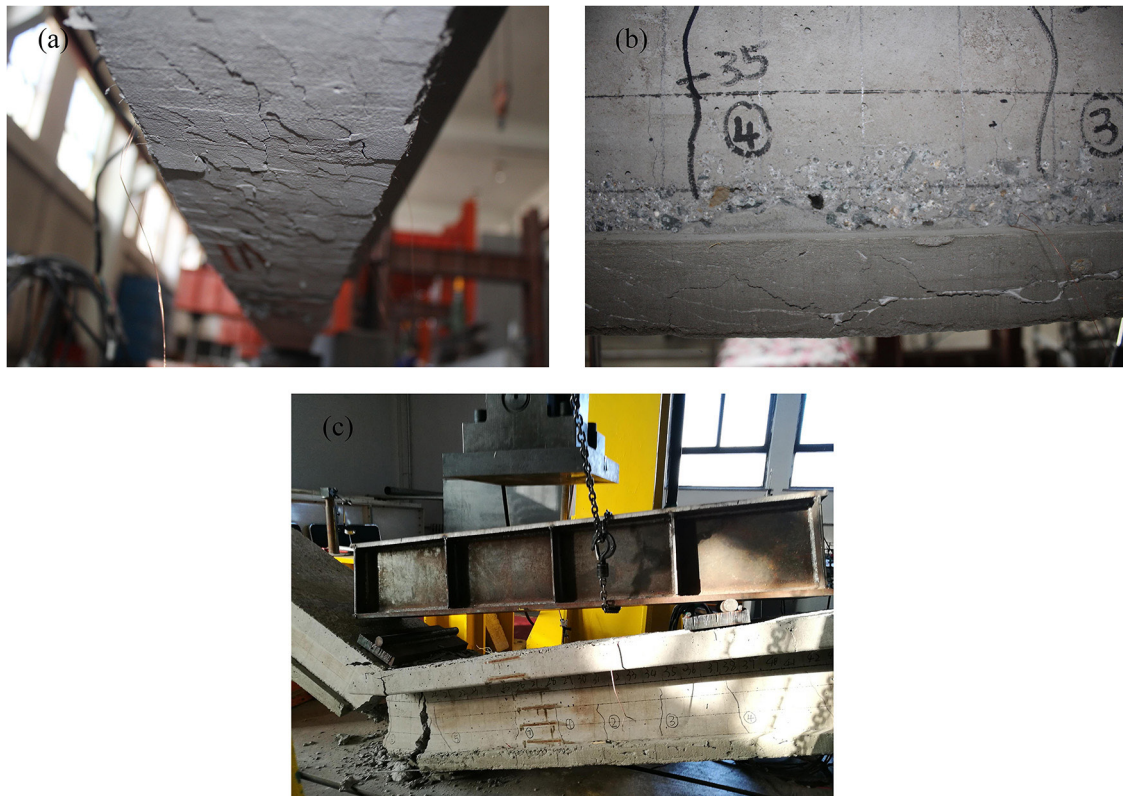
Figure 10: Midspan deflection and failure mode of beam PLB1 under fatigue load. (a) Cracking of polymer mortar; (b) Interlayer stripping of polymer mortar; (c) Steel bar fracture diagram of the beam PLB1.
