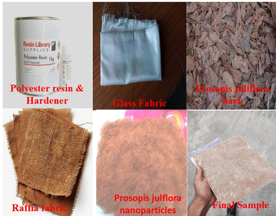
Figure 1: Materials used for prosopis juliflora reinforced bark nanoparticles hybrid composite.
