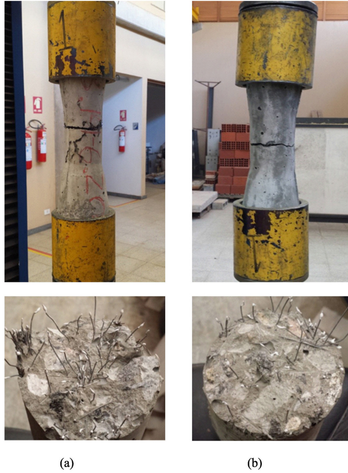
Figure 6: The failure of the specimens from the direct tensile test and the number of fibers ( N_f ) in the fractured plane. (a) Mixture F-15-2 ( N_f = 64.7 \pm 15.2 ); (b) mixture F-05-2 ( N_f = 24.3 \pm 10.0 ).
