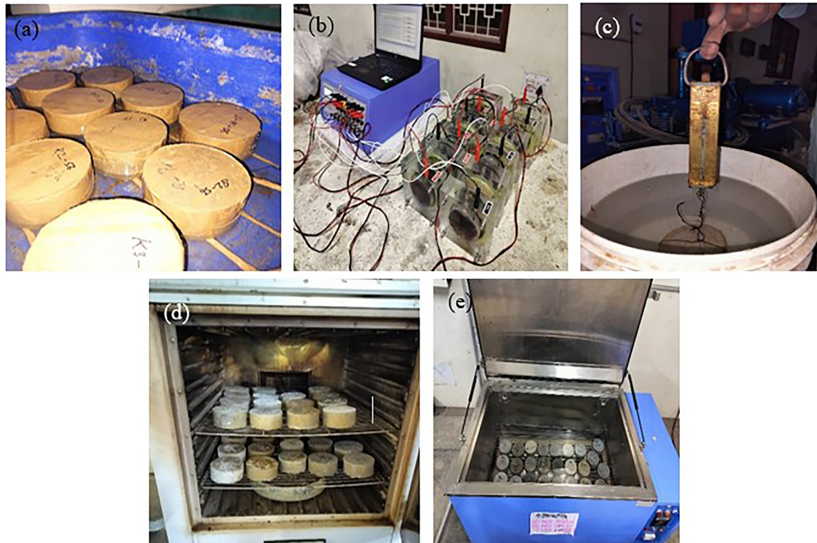
Figure 5: Experimental setup (a) sorptivity, (b) RCPT, (c) submerged specimens, (d) overdried specimens, (e) boiling specimens.
