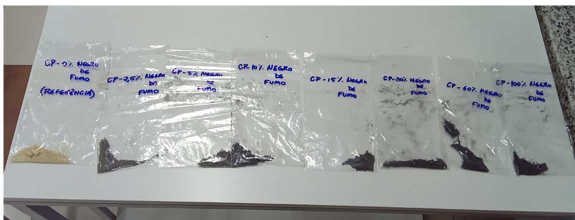
Figure 7: Samples for the FTIR test, where each plastic container contained 10 g of the powdered material and 3 test specimens in the form of 5 \times 5 cm plates with a flat surface.
