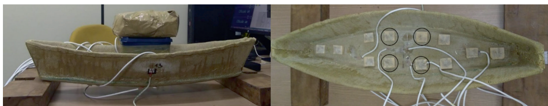
Figure 7: Internal loads and supports: internal load of 10 kg (left) load supports (right).
