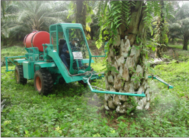
Figure 1 – Prototype prime mover with circle spraying attachment for spraying the palm circle.
