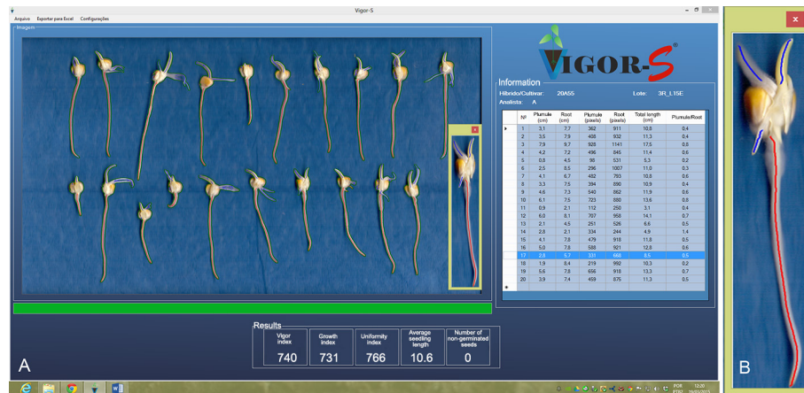
Figure 2 – Automated Analysis of Seed Vigor System – Vigor-S: analysis window showing a sample of scanned corn seedlings and processed by the software with results of vigor index (740), growth index (731), uniformity index (766), average seedling length (10.6 cm), number of non-germinated seeds (0) and table with the primary root length and total length of each seedling (A); detail of the seedling number 17 showing the primary root (red) and secondary roots and plumule (blue) (B).
