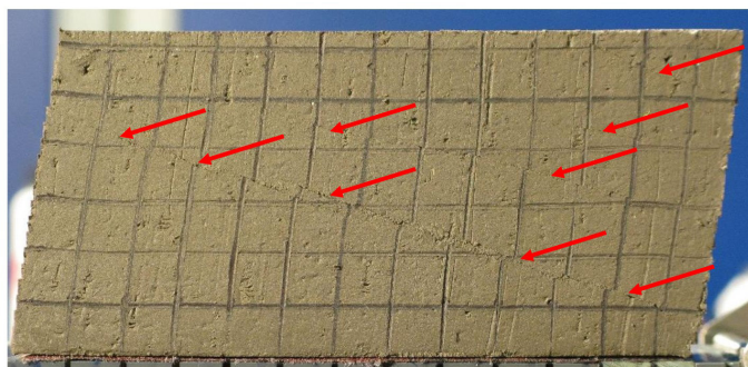
Figure 13. Results from a simple shear test on OVP clay sample ( \gamma = 20\% ) at the middle vertical plane (adapted from Grognet, 2011).
