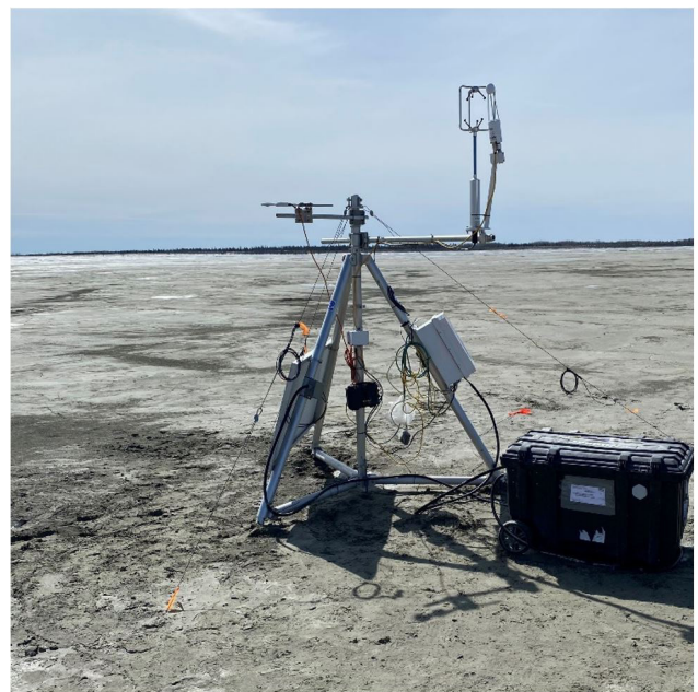
Figure 8. Eddy covariance instrumentation (ECV) on a tailings surface.
