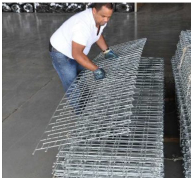
Figure 12. Closed articulated and galvanized formwork.
