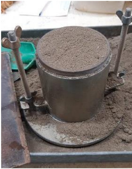
Figure 2. Moulded specimen for the Unconfined Compressive Strength Test (UCS).
