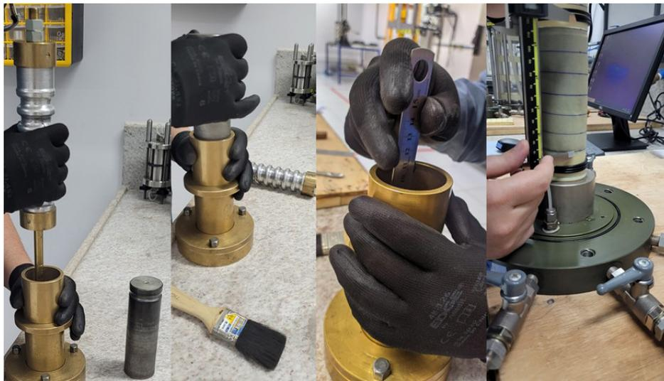
**Figure 4.** Dense specimen preparation method.
