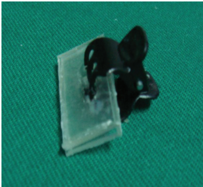
FIGURE 1 – Photograph of the compression device composed of transparent plastic plates affixed using a small claw equipped with a spiral spring that provides compression between the two plastic plates.
